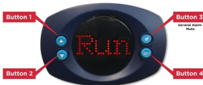
The Differential Pressure is factory set to 0.4 Bar. To reset the parameters (for example, the pressure differential) the following sequence needs to be followed on the VEXO® iX-2 Controller:
